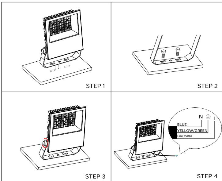
1. Drill holes on the installation surface as per bracket dimension diagram.
