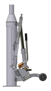
Hydraulic Counterbalance for Base Hinged Light Duty Columns - 4m - 8m
