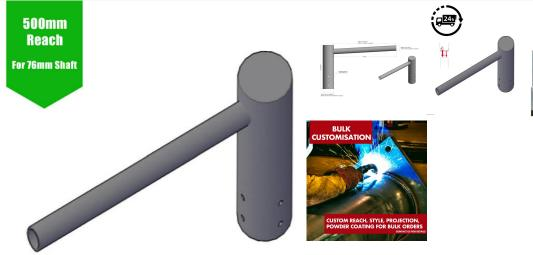
Lighting Column Arm - Single Projection Bracket 500mm Bracket - 60mm Arm Diameter - Steel Galvanised Post-Top for 76mm Shaft column entry. Supplied complete with 4 x M10 Grub screws for securing to the column shaft. **PLEASE NOTE - Weight & Windage must be checked for suitability of the bracket against the installation postcode. Please email us for more information prior to purchase.**
